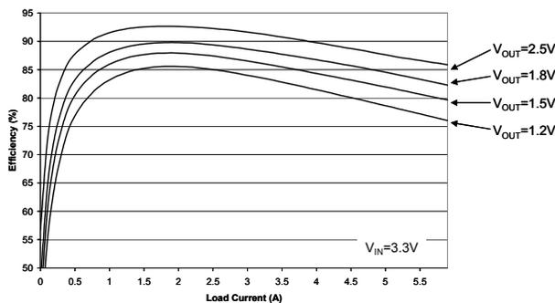
Efficiency vs. Load,  $V_{IN} = 3.3V$ .; Load = 0-6A.
