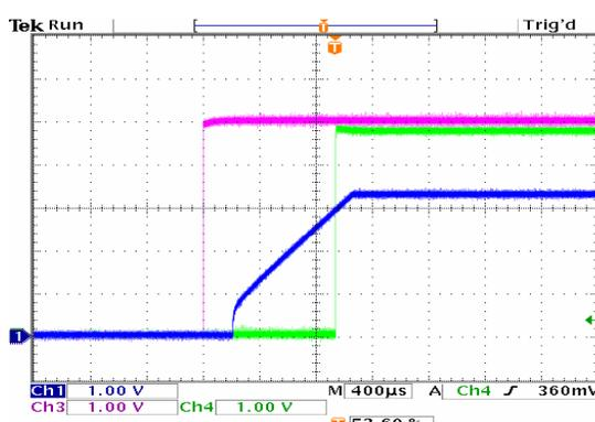
Start up waveforms V<sub>IN</sub>=5.0V, V<sub>OUT</sub>=3.3V, C<sub>SS</sub>=15nF,
