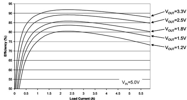
Efficiency vs. Load,  $V_{IN} = 5.0V$ .; Load = 0-6A.
