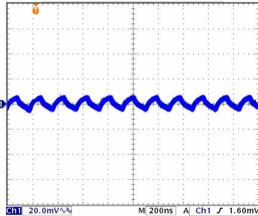
Ripple Voltage, 3.3V<sub>IN</sub>/1.2V<sub>OUT</sub>, I<sub>OUT</sub>=6A,
