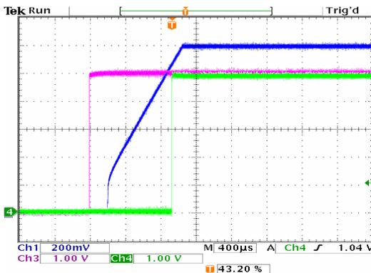
Start up waveforms V<sub>IN</sub>=5.0V, V<sub>OUT</sub>=1.2V, C<sub>SS</sub>=15nF,
