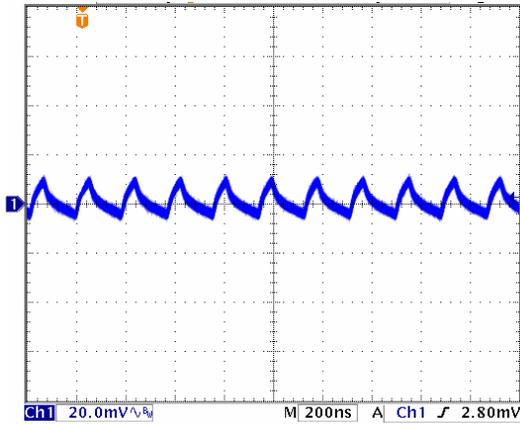
Ripple Voltage, 5.0V<sub>IN</sub>/1.2V<sub>OUT</sub>, I<sub>OUT</sub>=6A,
